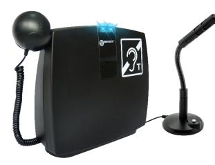
A portable unit designed for facilitating communication between a speaker and wearer/s of T-coil hearing aids. The LoopHEAR<sup>™</sup> is ideal for one to one applications such as at service counters, railway stations, banks, in vehicles and at small meeting rooms. This lightweight unit includes, within the casing an induction loop, a built-in amplifier and an external earpiece.
